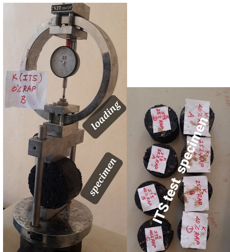
Figure 4 ITS test machine and test specimen respectively photo RRC central laboratory
