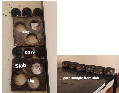
Figure 5 Core taking from lab compacted slab specimen (photo at RRC central laboratory)
