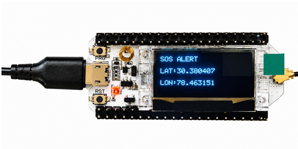
Fig. 4. Receiver/prototype module showing SOS and GPS information.
