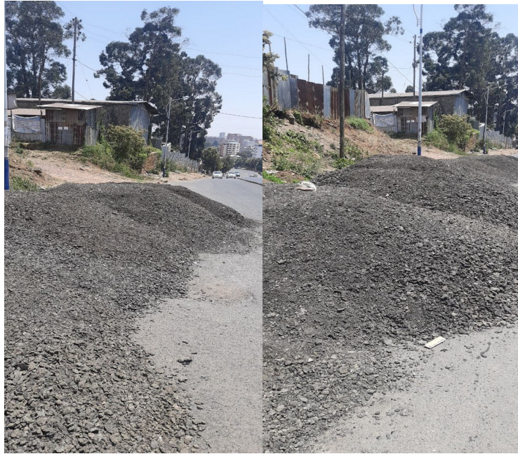
Figure 1 Source of RAP material from AACRA road project (photo taken during sampling)
