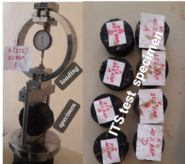
Figure 4 ITS test machine and test specimen respectively photo RRC central laboratory
