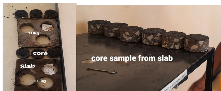
Figure 5 Core taking from lab compacted slab specimen (photo at RRC central laboratory)
